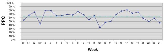
Figure 6: Percentage of Plan completed as function of time (calendar week)
