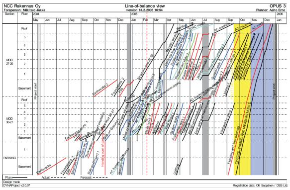
Figure 2: Master schedule of the Opus project—For clarity, only the construction and building services tasks which reserve the whole location are shown
