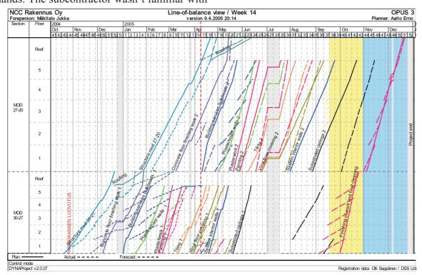
Figure 7: Actual situation (dotted lines) compared to the master schedule (solid lines). Forecasts based on the current task schedules are shown with dashed line.
