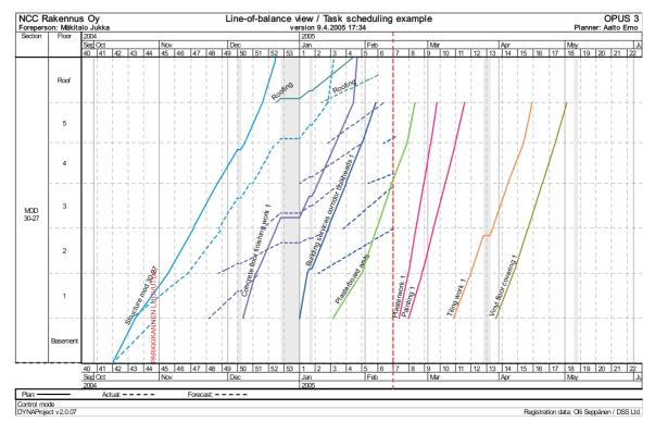
Figure 3: Original master schedule plan and actuals for plasterboard walls task and its predecessors and successors. Solid lines indicate the original plan, dotted lines the actual
