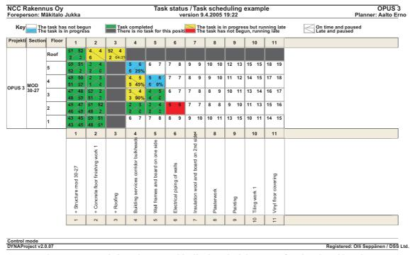
Figure 5: Control chart shows graphically the schedule status of each task and location
