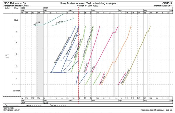
Figure 4: The task schedule for plasterboard walls task and its predecessors and successors
